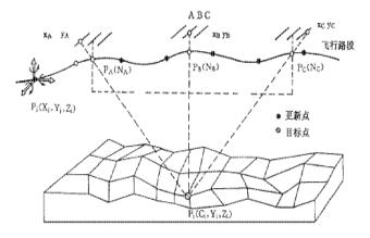
Figure 1 photogrammetry model of TLS CCD stereo surveying camera
